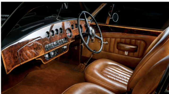
The interior of the Bensport Bentley La Sarthe is as opulent as it is classically British. Note that the original Bentley R-Type steering wheel has been used but that it has been reduced from 18" to 16" in diameter. The gear-lever is in the correct place for a classic Bentley also, on the right side. (Picture courtesy Bensport Ltd.)
