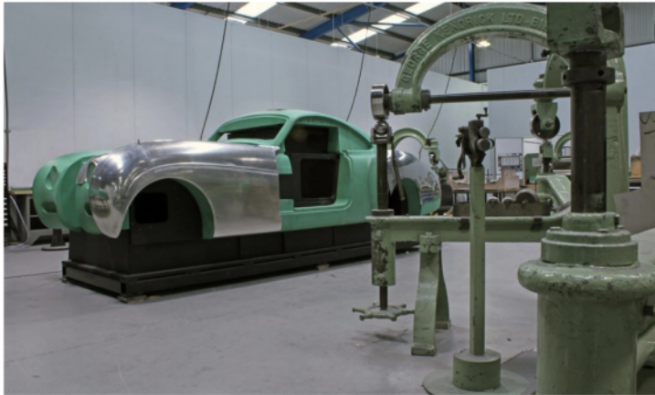
The bodywork of the La Sarthe is hand beaten aluminum. (Picture courtesy Bensport).
